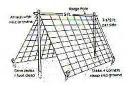
Drive support poles into ground about 1 foot as shown. Attach ridge pole of wood or metal, or stretch wire taut between support poles and extend it to ground (at an angel) at each end and secure with stakes.
